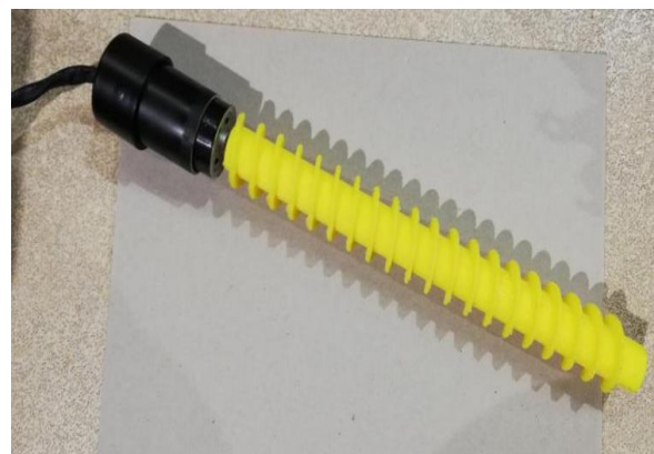
Fig. 4: Auger connected to a 12V DC Motor.
